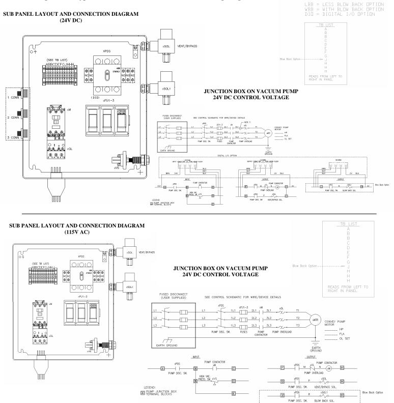
Figure 38: Typical SPDB 5-15 Series Junction Box Wiring Diagram
